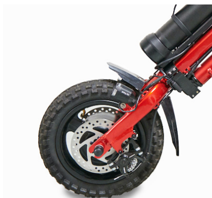
Dual disc brakes, dual lights and oversize 12.5" x 3" tire
