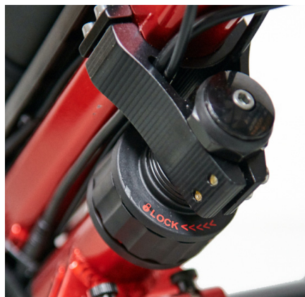
Locking headset for easier transfer & storage
