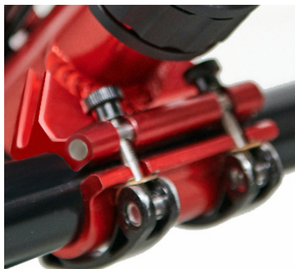
Frame easily comes apart via "Double quick release"
